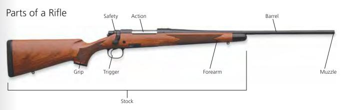
**Rifles** are designed to accurately hit a precise point. They are long-barreled firearms with grooves cut into the barrel of the rifle. These grooves are called rifling and give rifles their name. The rifling makes the bullet spin as it leaves the muzzle, making the projectile much more accurate and stable in flight. Make sure the ammunition you use matches the caliber that is stamped on the side of the barrel. You can find the caliber of the ammunition printed on the box.
