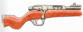
The bolt action is most often seen in rifles. Bolt action firearms are common and simple to use. Opening a bolt action firearm is as simple as pivoting the bolt upwards and pulling it backwards, using the handle on the bolt.
