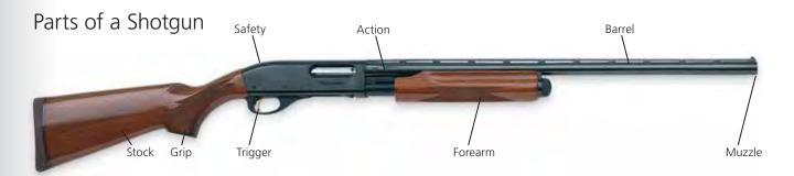
Shotguns typically shoot a spread of small projectiles instead of a rifle's single bullet. This increases the chances of hitting a moving target. They also have a smooth barrel inside. Shotgun styles allow a wide variety of choices including the gauge, the type of choke and the type of action. Shotguns can also fire a single projectile, called a slug, which is similar to a rifle bullet.
